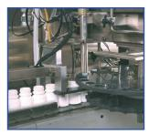
Süd-Chemie's canisters are ideal for high-speed insertion in pharmaceutical and nutraceutical packaging.
